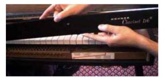
Remove the front panel by pulling down on its top ledge, it is partially seated in a notch on the left wood panel and it sits below the right wood panel.
