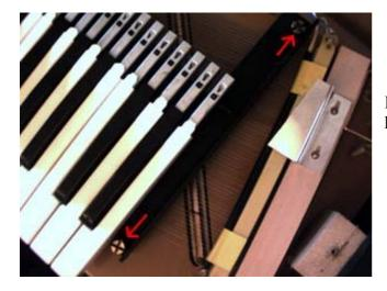
Locate the two screws on the right side of the keyboard assembly and remove.
