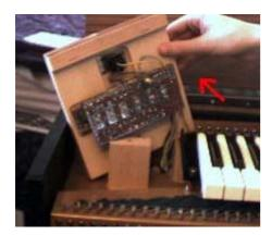
Since the left wood panel is electrically attached to the keyboard, simply set it behind the wood block standing up.
